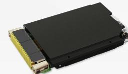
Renice 3U Open VPX SATA memory card adapt dual-channel SATAIII protocol, built-in military SSD, the single SATA sequential Read/Write is more than 500MB/s and the maximum capacity able to support 10TB. It is suitable for the data storage in the application of industry and military, especially for high impact and high vibration environment.
